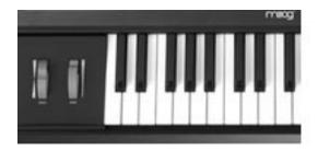
The Little Phatty has a 37-note keyboard (3 octaves, C to C). When combined with the **OCTAVE** buttons, the keyboard has a playable range of 7 octaves. The keyboard produces velocity control voltages and transmits MIDI Note On and Note Off messages polyphonically. To the left of the keyboard is the Left Hand Controller Panel, which contain the Pitch Bend and Mod Wheel controls.
