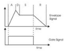
The second auxiliary component is the Envelope Generator, or EG. The EG makes no sound by itself. Rather, it creates a time-varying control voltage that is typically used to control the gain of the amplifier, or the cutoff frequency of the filter. Many synthesizers, including the Little Phatty, provide several EG's for independent envelope control of the amplifier and filter circuits.
