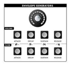
The Little Phatty has two identical EG circuits. When triggered, these circuits produce time-varying control voltages having a start, middle and an end. The parameters that specify this progression are the Attack, Decay, Sustain and Release controls, sometimes abbreviated as ADSR.
