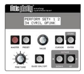
To enter master mode, press the **MASTER** button. By default, the first master menu entry is Performance Sets. When switching between the Master and Preset modes, the last used master menu entry appears.
