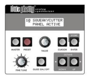
Preset sounds are selected using the **VALUE** knob. As the **VALUE** knob is advanced, the next preset appears in the display and is immediately available to be auditioned (you do not need to 'activate' the preset to hear it). Pressing **VALUE** and turning the knob will advance by increments of ten.
