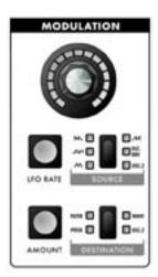
Modulation is the heart of making interesting sounds with analog subtractive synthesis. The LP's Modulation section opens up a world of modulation possibilities that were not available on the original Minimoog. The Modulation section allows you to select from six modulation sources, four destinations, and set the modulation amount. The output of the Modulation section is controlled by the Modulation Wheel.
