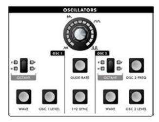
Oscillator One serves as a master oscillator to which Oscillator 2 is tuned. The timbres of the oscillators are adjusted by their variable waveform (Wave) controls. There is also a switch for syncing Oscillator 2 to Oscillator 1, and a control for adjusting the glide rate which is explained below.
