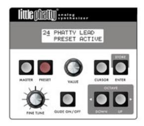
The status display is an LCD screen located in the center of the panel above the section controls. When the LP is first powered on, the screen will display the message:
