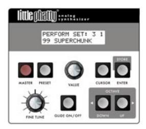
The example on the right shows the preset stored in the first location of Performance Set 3 (Preset 99 – SUPERCHUNK). To step through this sequence, press the **VALUE** switch. Each press will advance to the next preset in the sequence. After the eighth preset is reached, the next press of the **VALUE** switch will cycle back to the first preset in Performance Set 3.
